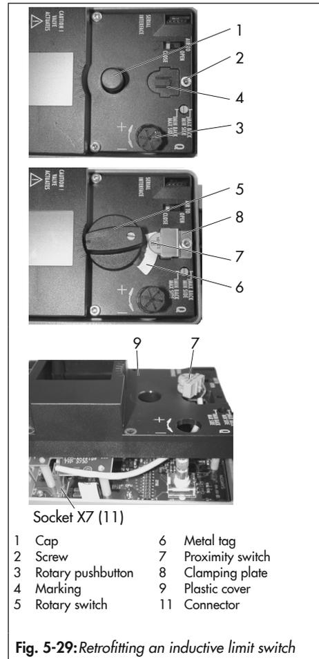
**Fig. 5-29:** Retrofitting an inductive limit switch
