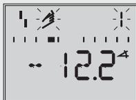
After *tESinG* runs across the display, the **⚡** fault alarm icon appears and the **✋** hand icon blinks on the display when the **positioner has not been initialized**. The reading indicates the lever position in degrees in relation to the mid-axis.
