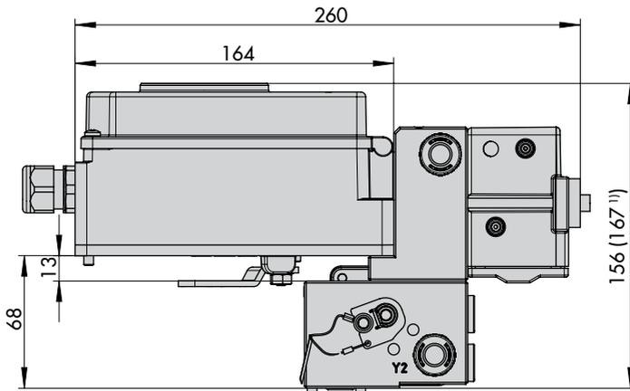
Attachment to rotary actuators according to VDI/VDE 3845
