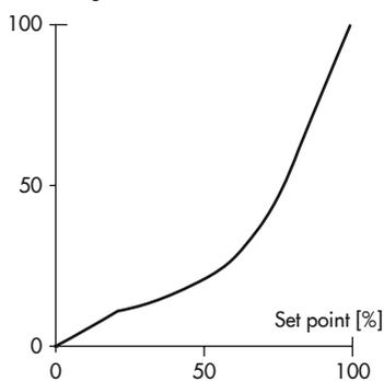
**Segmented valve ball linear** (select characteristic: 7)
