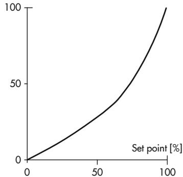
**VETEC rotary plug valve linear** (select characteristic: 5)
