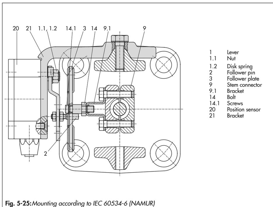
Fig. 5-25: Mounting according to IEC 60534-6 (NAMUR)
