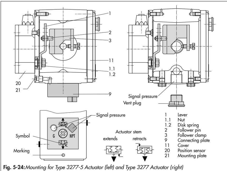
Fig. 5-24: Mounting for Type 3277-5 Actuator (left) and Type 3277 Actuator (right)
