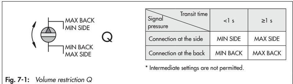
The volume restriction Q serves to adapt the air output capacity to the size of the actuator:
