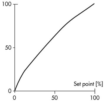
**VETEC rotary plug valve equal percentage**
