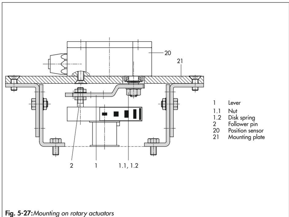
Fig. 5-27: Mounting on rotary actuators
