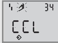
Closing direction (direction of rotation causing the valve to move to the CLOSED position (view onto positioner display); standard CCL
