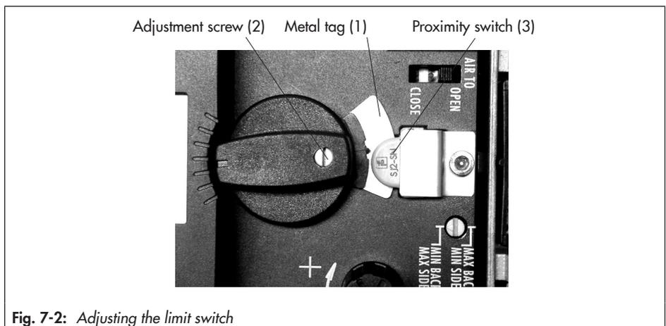
Fig. 7-2: Adjusting the limit switch
