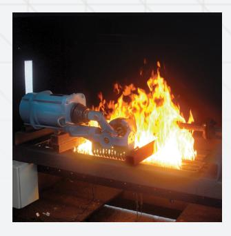
**SOLUTION:** The 82.7 is fire-safe certified according to API 607 and ISO 10497 for use in these areas.
